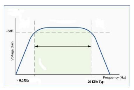
Fig. 2 Typical Bode Plot for EPIC ECG Sensor
