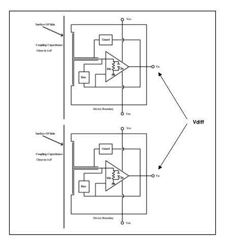
Fig. 3 Differential measurement of body (skin) surface potential to produce ECG trace
