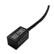
The Model 52M32 accelerometer has an advanced piezoresistive MEMS sensing element which offers excellent dynamic range and stability. This unit features a full bridge output with an operating temperature range from -40 to +90°C. A slight amount of gas damping provides outstanding shock survivability and a flat amplitude response to 6kHz.
