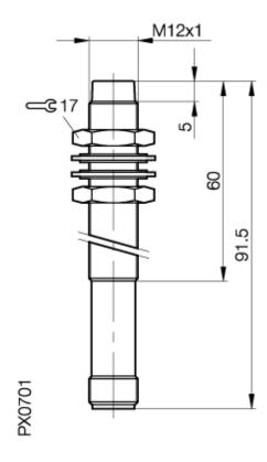
**Inductive Sensors** BES 113-356-SA 6-S 4 M12x1 x 91.5 normally-open **Sn=3,7mm** unshielded function monitoring
