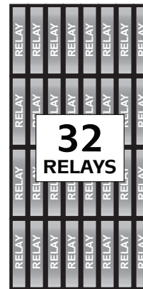
Using PICKERING Series 109 relays in this PCB area you can fit 32 Relays
