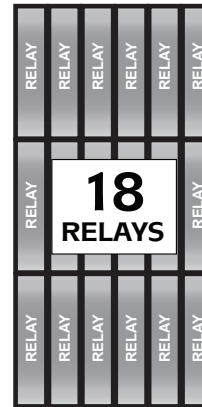
Using standard 0.2 x 0.8 inch relays in this PCB area you can fit 18 Relays
