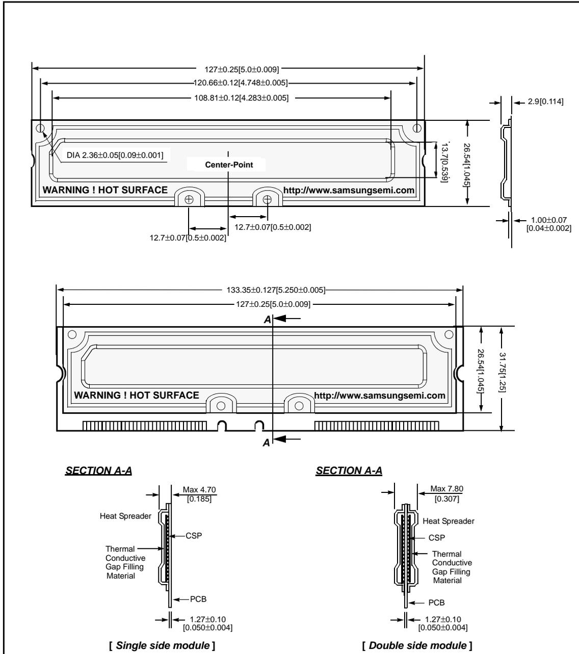
Figure 5: Heat Spreader Physical Dimensions
