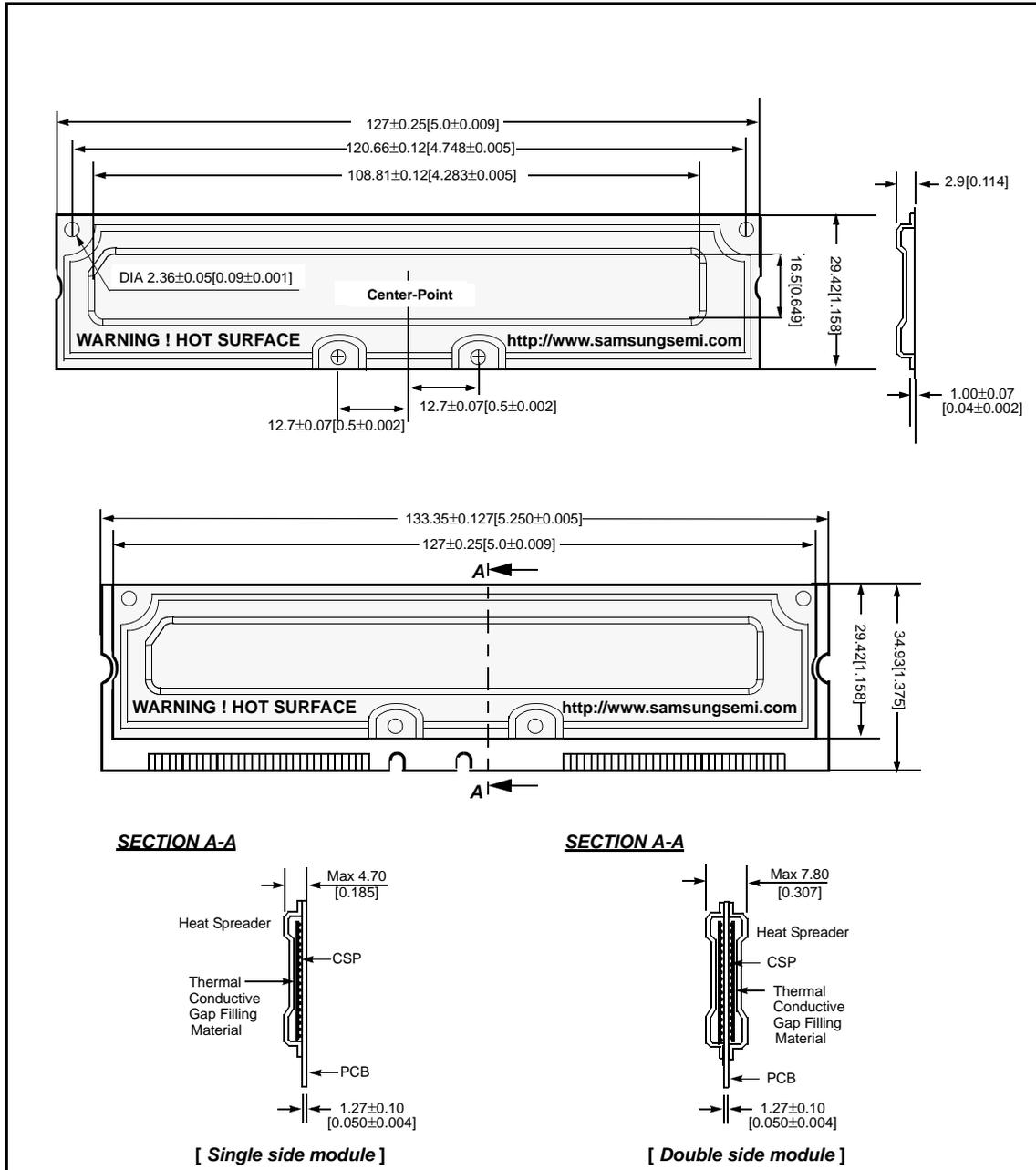
Figure 6: Heat Spreader Physical Dimensions
