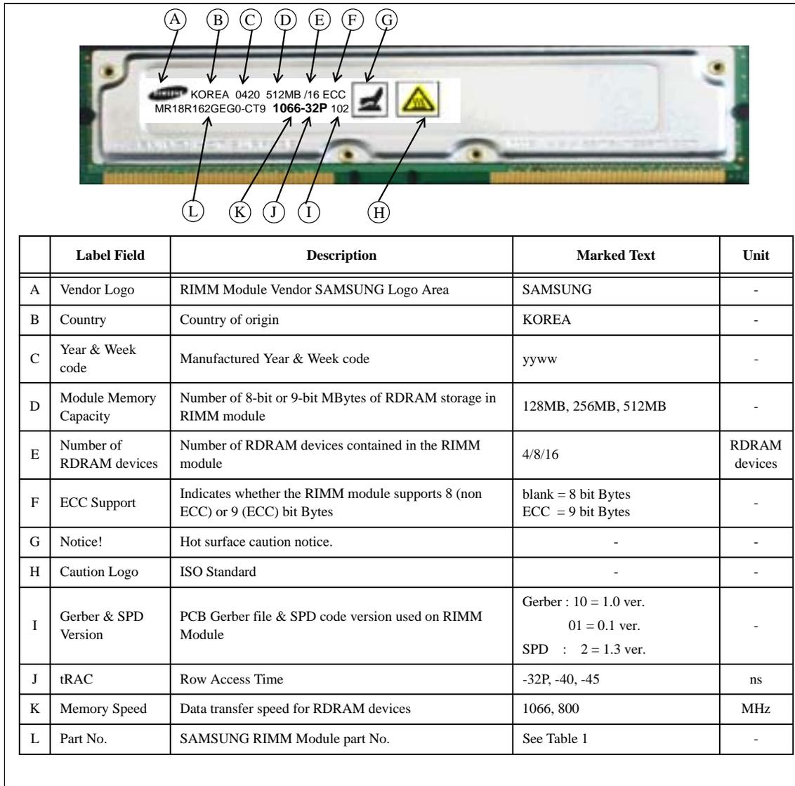
Figure 7: RIMM Module Marking Example
