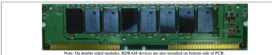
Note: On double sided modules, RDRAM devices are also installed on bottom side of PCB.
