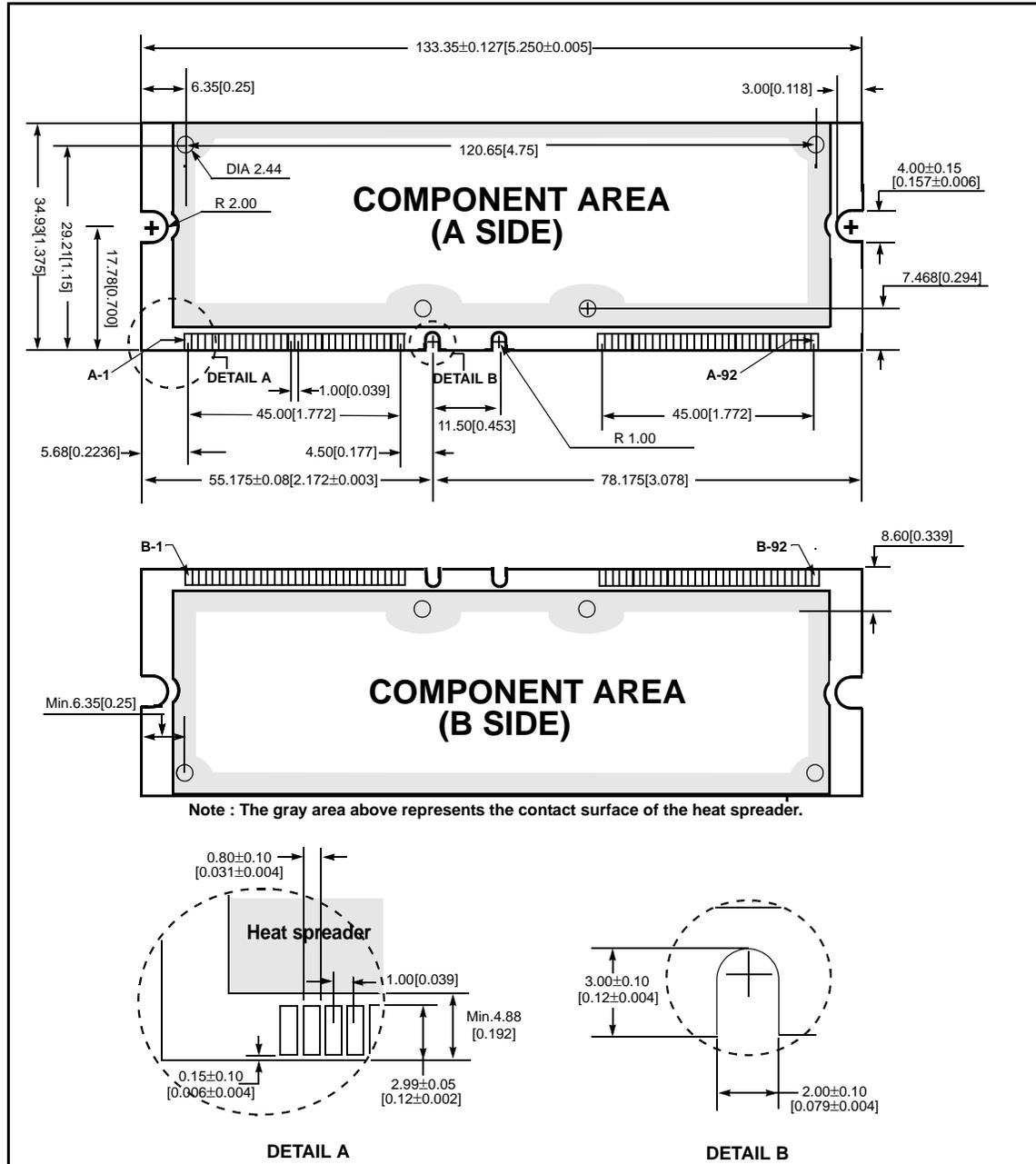
Figure 4: 256Mb/288Mb base RIMM Module PCB Physical Dimensions
