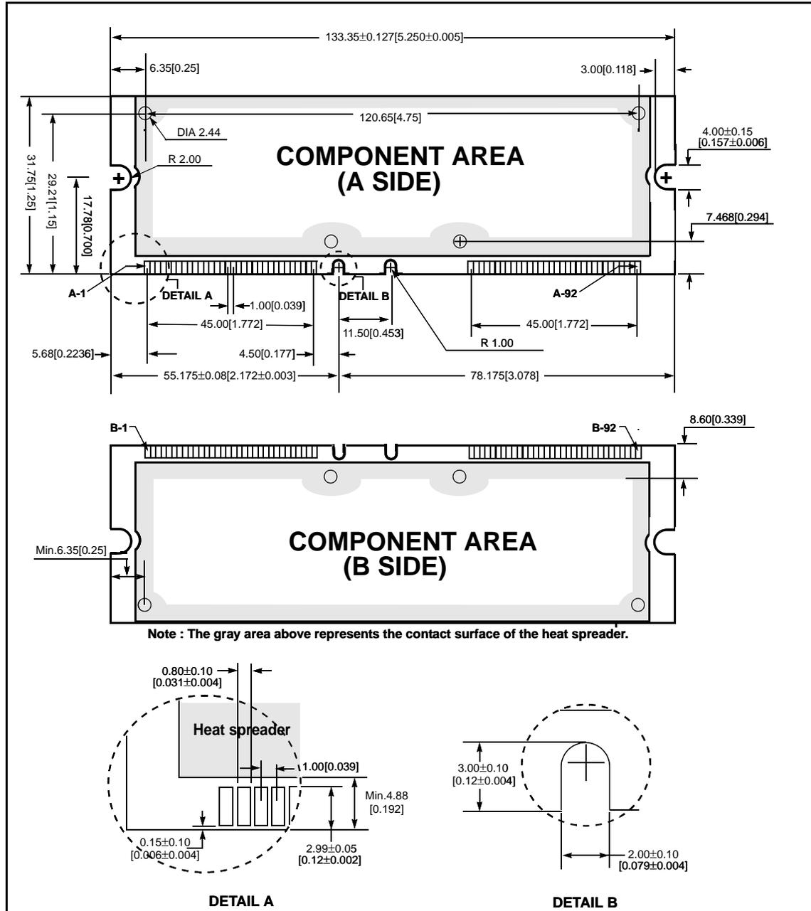
Figure 3: 256Mb/288Mb base RIMM Module PCB Physical Dimensions
