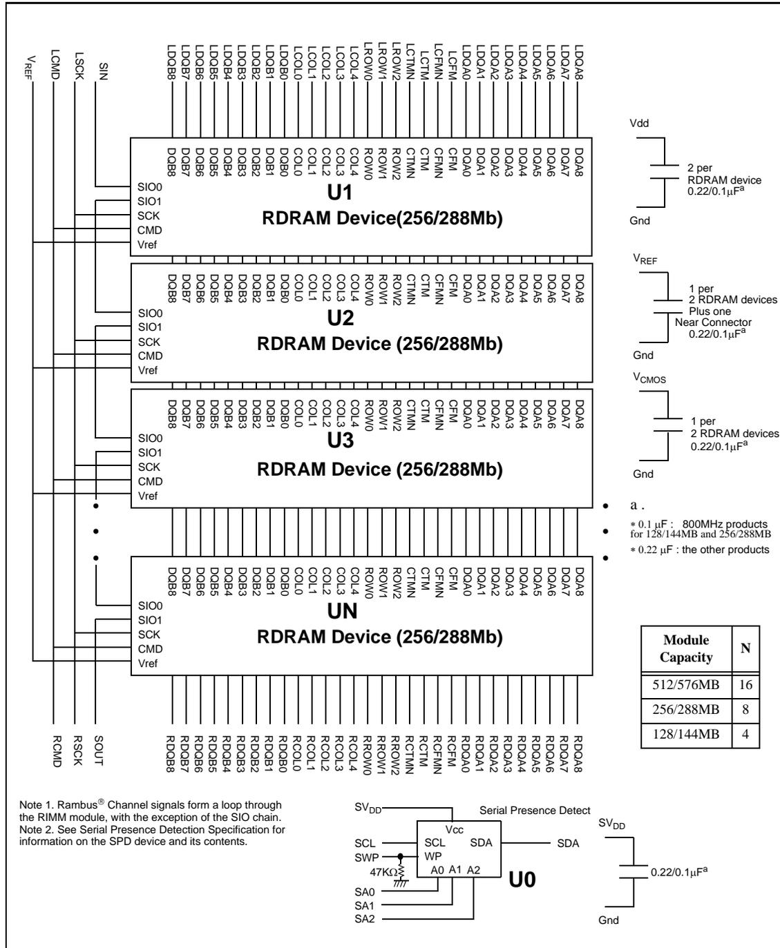
Figure 2: RIMM Module Functional Diagram
