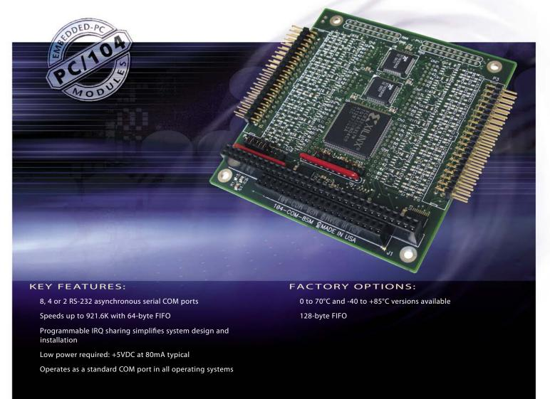
The 104-COM232-8 series are eight, four, or two-port asynchronous, RS-232 serial communication boards. The boards are feature-rich and allow for the connection of multiple serial devices—ideal for a variety of applications such as POS, barcode readers, modems, machine monitoring and control, military, high-density networking applications or any other application requiring the connection of RS-232 serial devices to a PC/104 compatible system.
