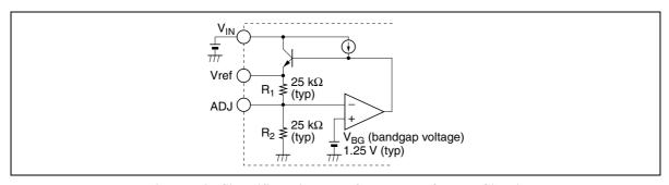
Figure 5.2 Simplified Diagram of Voltage Reference Circuit
