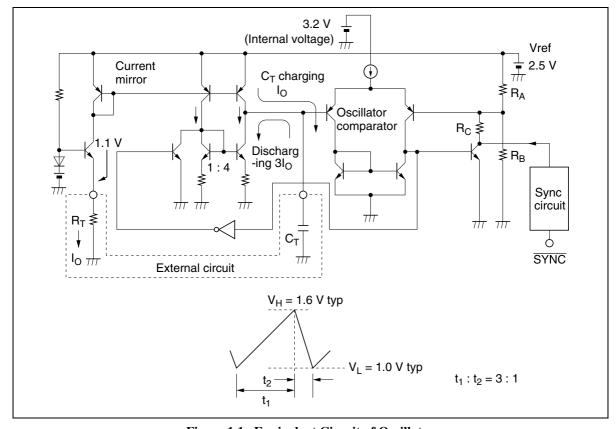
Figure 1.1 Equivalent Circuit of Oscillator
