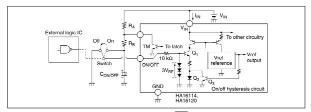
Figure 6.1 Shutdown by ON/OFF Pin Control
