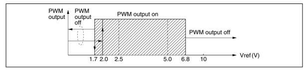
Figure 5.4 Vref Undervoltage Lockout and Overvoltage Protection
