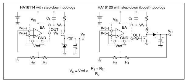
Figure 2.1 Output Voltage Setting (1)
