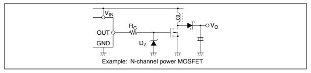
Figure 4.2 Gate Protection by Zener Diodes
