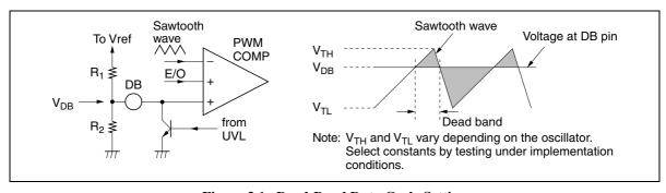
Figure 3.1 Dead-Band Duty Cycle Setting
