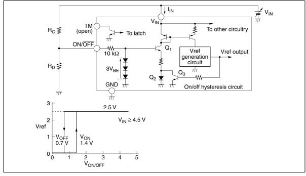
Figure 6.2 Adjustment of UVL Voltages
