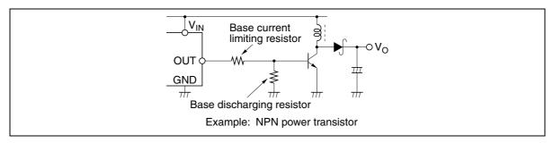
Figure 4.3 Driving a Bipolar Power Transistor
