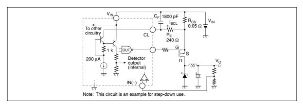
Figure 8.1 Example for Step-Down Use
