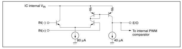
Figure 2.3 Error Amplifier Equivalent Circuit
