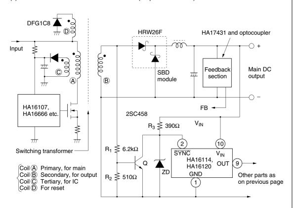
This circuit illustrates the combination of the HA16114/120 with a forward AC/DC converter. The HA16114/120 synchronizes with the falling edge of the external sync signal, so with a forward transformer, the sync pulses must be inverted. In the diagram, this is done by an external circuit consisting of the following components:
