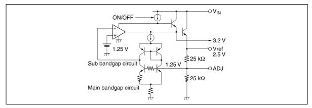
Figure 5.1 Vref Reference Circuit
