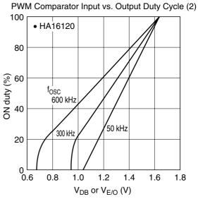
Note: The on-duty of the HA16120 is the proportion of one cycle during which output is high.
