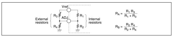
Figure 5.3 Trimming of Reference Voltage
