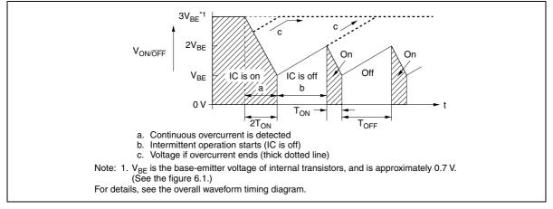
Figure 7.2 Intermittent Mode Timing Diagram (V<sub>ONOFF</sub> only)
