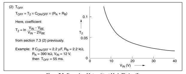
Figure 7.5 Examples of Intermittent Mode Timing (2)
