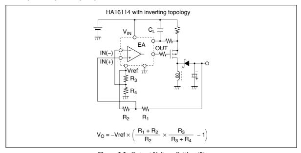
Figure 2.2 Output Voltage Setting (2)
