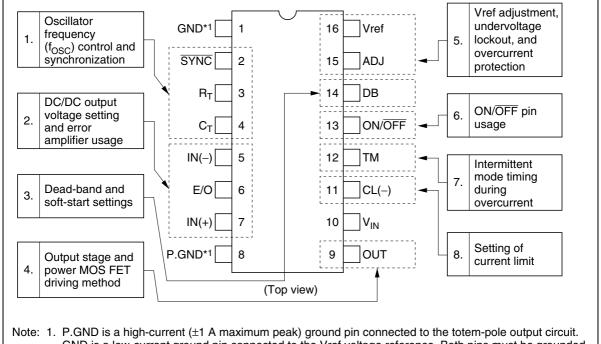
GND is a low-current (±1 A maximum peak) ground pin connected to the totem-pole output circuit.
