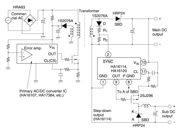
This is one example of a circuit that uses the features of the HA16114/120 by operating in synchronization with a flyback AC/DC converter. Note the following design points concerning the circuit from the secondary side of the transformer to the SYNC pin of the HA16114/120.
