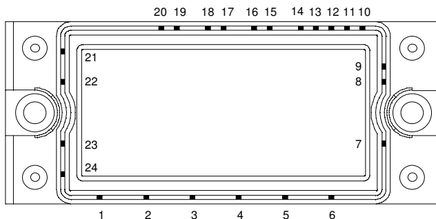
APTGF30X60RTP2: Without Brake (Pin 7 & 14 not connected)
