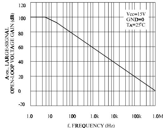
Figure 2. Open-Loop Frequency
