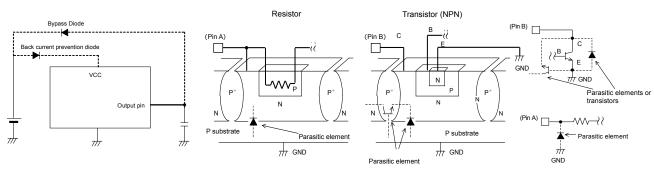
Fig. 22 Example of Simple Bipolar IC Architecture
