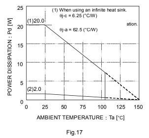
The characteristics of the IC are greatly influenced by the operating temperature. If the temperature exceeds the maximum junction temperature T<sub>jmax</sub>, deterioration or damage may occur. Implement proper thermal designs to ensure that power dissipation is within the permissible range in order to prevent instantaneous damage resulting from heat and maintain the reliability of the IC for long-term operation.
