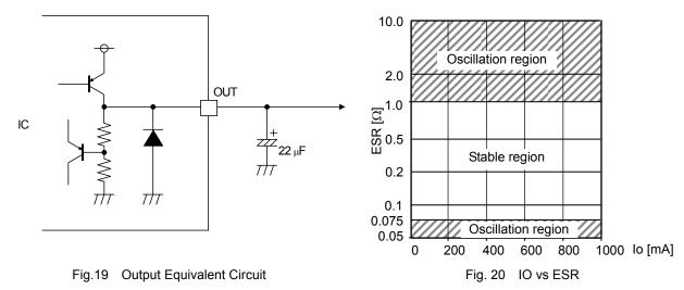
The capacitance may vary greatly with temperature changes, thus making it impossible to completely prevent oscillation. Therefore, use a tantalum aluminum electrolytic capacitor with a low ESR (Equivalent Serial Resistance). The output will oscillate if the ESR is too high or too low, so refer to the ESR characteristics in Fig. 20 and operate the IC within the stable region. Use a capacitor within a capacitance between  $22\mu$ F and  $1,000\mu$ F.
