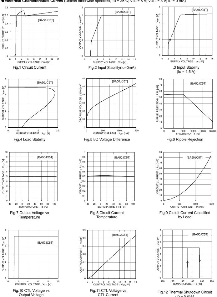
Fig.12 Thermal Shutdown Circuit (Io = 5 mA)
