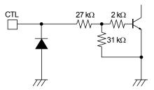
Fig.18 Input Equivalent Circuit
