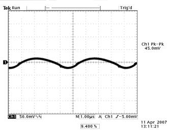
Photo 8: Output Ripple and Noise (20 MHz BW) Vin=24 V, Iout = 2.5 A With a 22 uF Tantalum across the Output
