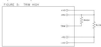
NOTE 1: CONNECT TRIM RESISTOR AS CLOSE TO CONVERTER PINS AS POSSIBLE
