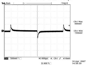
**Photo 10:** Transient Response – 0.1 A/us Vin=24 V, Iout = 1 to 3 A (25% to 75%)
