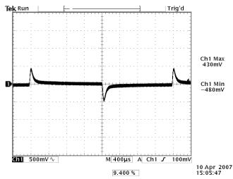
Photo 11: Transient Response – 0.1A/us Vin=24 V, Iout = 1 to 3 A (25% to 75%) With a 22 uF Tantalum across the Output
