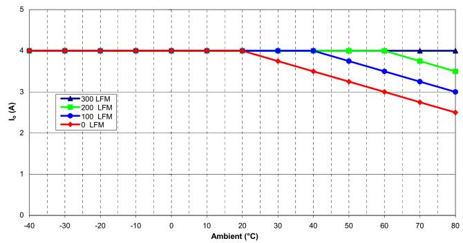
**Note 3:** When trimming output high, I<sub>o</sub> vs. Ambient is derated by power. ie: from Graph 2, find the maximum current at the desired ambient and airflow, and multiply this current by the nominal voltage to get the maximum power. Divide this power by the desired trimmed high voltage to get the maximum current at that ambient. When trimming low, the maximum current stays the same as shown in Graph 2.
