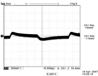
**Photo 9:** Transient Response – 0.01 A/us Vin=24 V, Iout = 1 to 3 A (25% to 75%)
