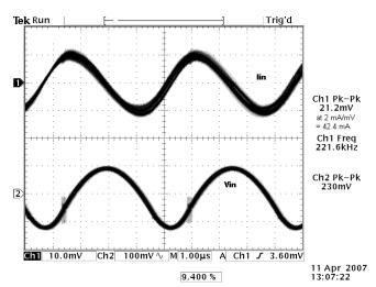
Photo 2: Input Ripple Voltage and Current Vin=24 V, Iout = 4 A
