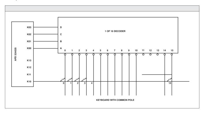
To scan more than 16 switches, a 4 line to 16 line decoder must be added, which will allow scanning up to 64 keys. In this mode the keyboard outputs (KO0-KO3) will work as a 4 bit binary counter.
