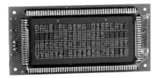
The APD-080M025-1 plasma display module consists of a multiplexed DC plasma display, drive circuitry and switching voltage converter mated with an intelligent, microprocessor-based controller board. The resulting assembly interfaces easily to microprocessor based systems and only requires readily available low voltages for power. Vishay Dale's patented open construction display technology assures a stable flicker free screen even at highest communication rates.
