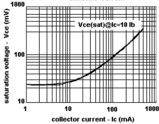
**Figure 3. Saturation Voltage vs Collector Current**
