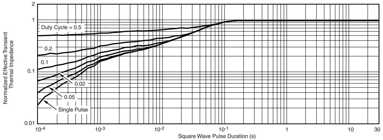
Normalized Thermal Transient Impedance, Junction-to-Case
