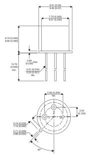
Bipolar NPN Device in a Hermetically sealed TO39 Metal Package.
