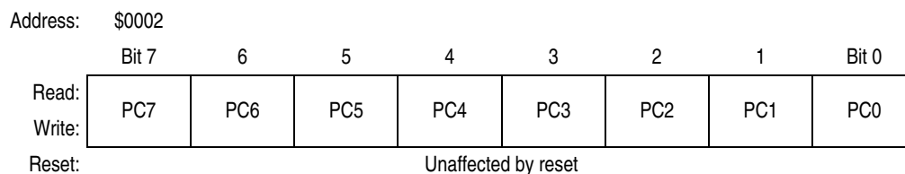
Figure 6-5. Port C Data Register (PORTC)
