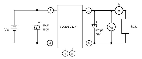
It is used the electrolytic capacitors which has the low impedance for output capacitor.
