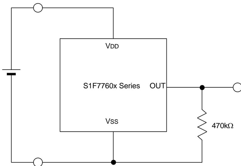
This explanatory diagram covers a P-ch open drain output model.
