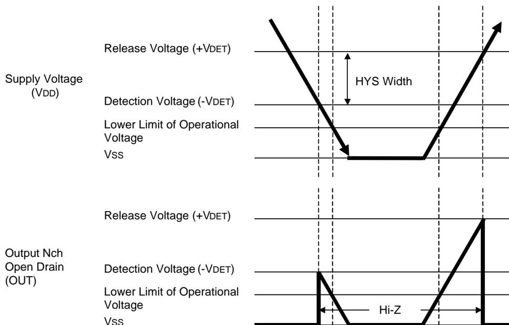
Fig.7.1.2 I/O characteristics of N-ch open drain
