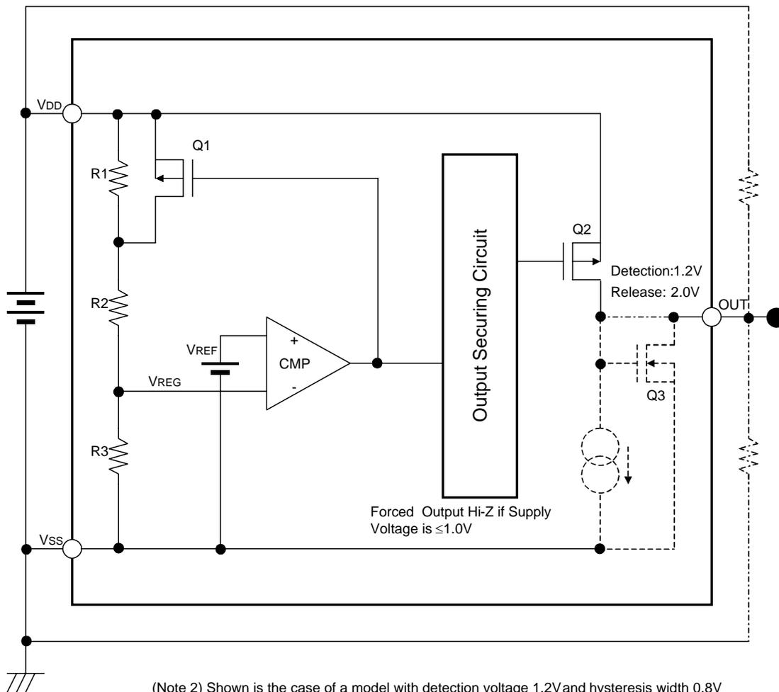
(Note 2) Shown is the case of a model with detection voltage 1.2V and hysteresis width 0.8V
