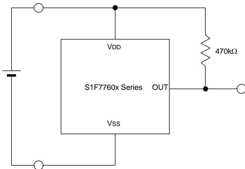
This explanatory diagram covers an N-ch open drain output model.
