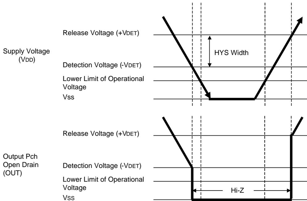
Fig.7.1.1 I/O characteristics of P-ch open drain
