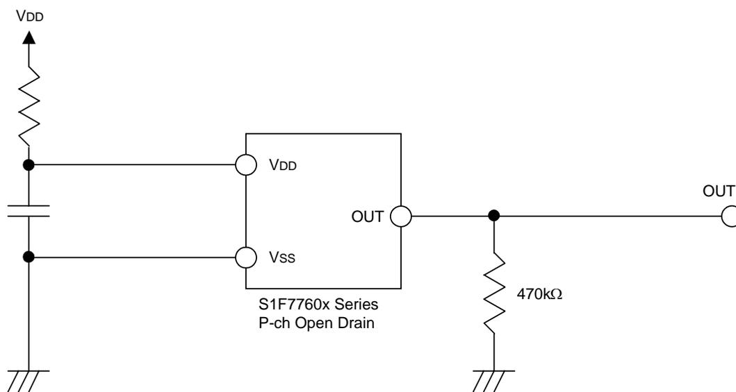
Fig.11.3 Example of circuit 3 (CR timer circuit)
