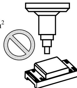
Failure to comply might result in damage to encapsulant and in the worst cases, catastrophic failure of the LEDs due to wire deformation and/or breakage.
