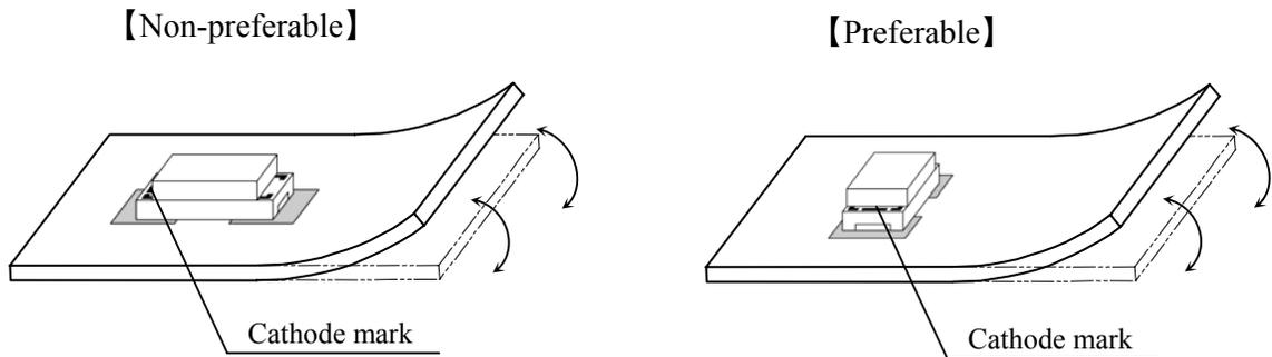
When mechanical stress from the board affects the soldered LED, place the LED in the preferable location and orientation as shown above.
