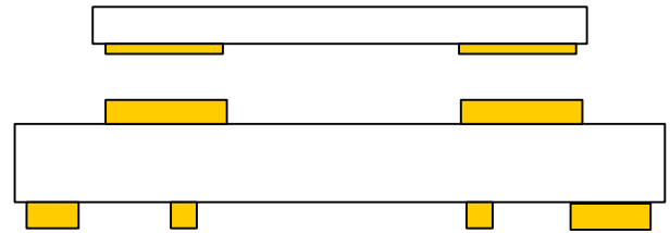
Figure 21. Correct PCB Top Metal Pattern Under Package
