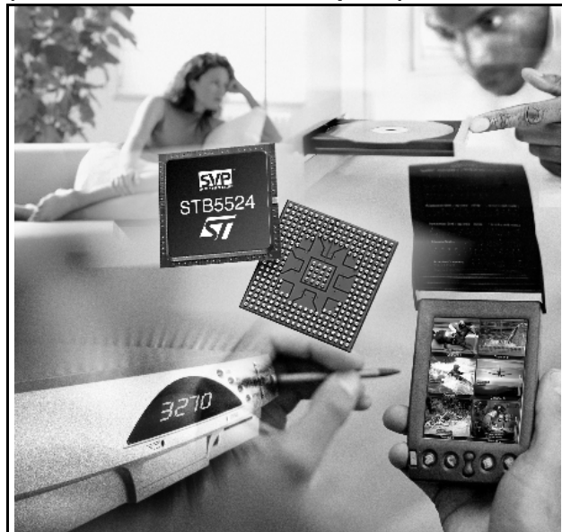
Figure 1. Package (27 x 27 PGBGA 416, 1 mm pitch)
