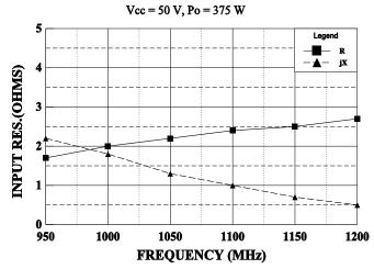
SERIES LOAD IMPEDANCE vs FREQUENCY
