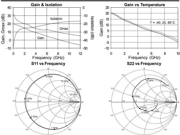
Note: S-parameters are de-embedded to the device leads with  $Z_s = Z_L = 50\Omega$ . The data represents typical performace of the device. De-embedded s-parameters can be downloaded from our website (www.sirenza.com).
