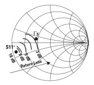
Figure 1. Input Match for ATF-521P8 at 2 GHz.
