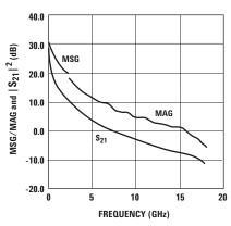
Figure 41. MSG/MAG and  $|S_{21}|^2$  vs. Frequency at 4.5V, 200 mA.
