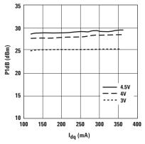
Figure 11. P1dB vs.  $I_{dq}$  and  $V_{ds}$  at 2 GHz.
