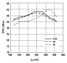
Figure 10. OIP3 vs.  $I_{ds}$  and  $V_{ds}$  at 3.9 GHz.
