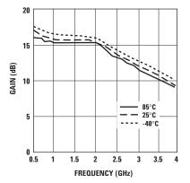
Figure 22. Gain vs. Temp and Freq tuned for optimal OIP3 at 4.5V, 200 mA.
