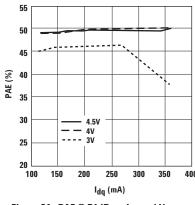
Figure 34. PAE @ P1dB vs.  $I_{dq}$  and  $V_{ds}$  at 900 MHz.
