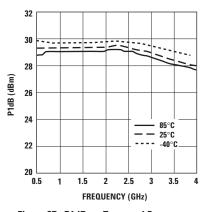
Figure 37. P1dB vs. Temp and Freq (tuned for optimal P1dB at 4.5V, 200 mA).
