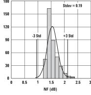
Figure 2. NF @ 2 GHz, 4.5 V, 200 mA. Nominal = 1.5 dB.
