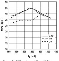
Figure 8. OIP3 vs.  $I_{ds}$  and  $V_{ds}$  at 2 GHz.
