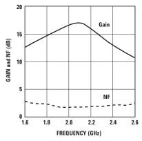
Figure 15. Gain and Noise Figure vs. Frequency.
