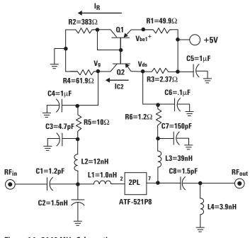
Figure 14. 2140 MHz Schematic.
