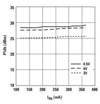
Figure 29. P1dB vs.  $I_{dq}$  and  $V_{ds}$  at 3.9 GHz.
