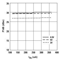
Figure 27. P1dB vs.  $I_{dq}$  and  $V_{ds}$  at 2 GHz.
