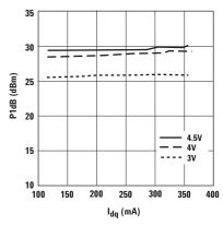
Figure 28. P1dB vs.  $I_{\mbox{\scriptsize dq}}$  and  $V_{\mbox{\scriptsize ds}}$  at 900 MHz.
