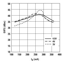
Figure 26. OIP3 vs.  $I_{ds}$  and  $V_{ds}$  at 3.9 GHz.
