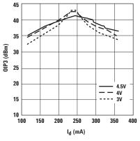
Figure 24. OIP3 vs.  $I_{ds}$  and  $V_{ds}$  at 2 GHz.
