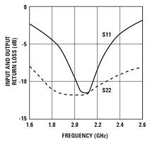
Figure 16. Input and Output Return Loss vs. Frequency.
