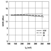
Figure 30. Gain vs  $I_{ds}$  and  $V_{ds}$  at 2 GHz.
