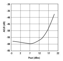
Figure 18. ACLR vs. Pout at 5 MHz Offset.
