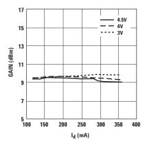
Figure 32. Gain vs  $I_{ds}$  and  $V_{ds}$  at 3.9 GHz.
