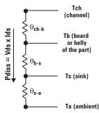
Figure 19. Equivalent Circuit for Thermal Resistance.
