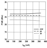
Figure 12. P1dB vs.  $I_{\mbox{\scriptsize dq}}$  and  $\mbox{\scriptsize V}_{\mbox{\scriptsize ds}}$  at 900 MHz.
