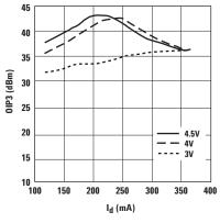
Figure 9. OIP3 vs.  $I_{ds}$  and  $V_{ds}$  at 900 MHz.
