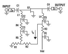
Figure 8. Passive Biasing.
