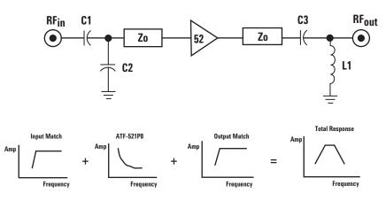
Figure 7. Input and Output Match for ATF-521P8 at 2 GHz.
