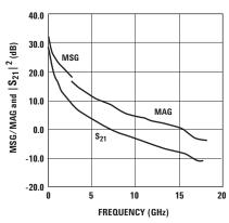
Figure 42. MSG/MAG and  $|S_{21}|^2$  vs. Frequency at 4.5V, 120 mA.
