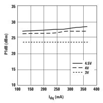
Figure 13. P1dB vs.  $I_{\mbox{\scriptsize dq}}$  and  $V_{\mbox{\scriptsize ds}}$  at 3.9 GHz.
