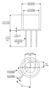
Bipolar PNP Device in a Hermetically sealed TO39 Metal Package.
