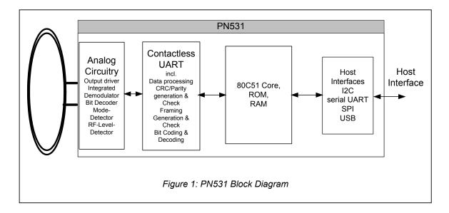
The Analog circuitry handles the modulation and demodulation of the analog signals according to the card mode, reader /writer mode and NFC mode communication scheme.
