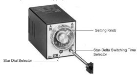
The scale range on the star side can be selected from four different ranges of 0 to 5, 0 to 10, 0 to 50, and 0 to 100 displayed in the six windows by turning the Star Dial Selector. Note that the selectors does not turn infinitely.
