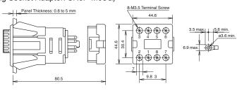
(11-pin Screw Terminal Wiring Socket Adapter: SR6P-M11G)
