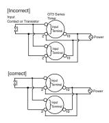
In a transistor circuit for controlling input signals with its primary and secondary power circuits isolated, do not ground the secondary circuit.
