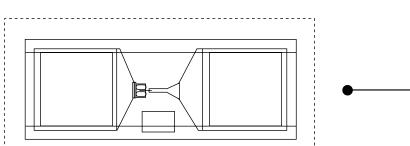
Chip Size: Chip Size Tolerance: Chip Thickness: Chip Thickness Tol: Bond Pad Sizes: 610 x 255 µm (24 x 10 mils) ±10 µm (±0.4 mils) 100 µm (4 mils) ±15 µm (±0.6 mils) 175 x 175 µm (6.9 x 6.9 mils)
