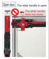
If the lockout key is not mounted, the slide handle will not move and the door will not close.
