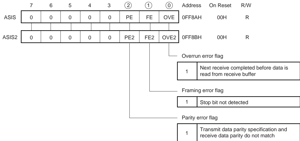
Figure 16-4 Format of Asynchronous Serial Interface Status Register (ASIS) and Asynchronous Serial Interface Status Register 2 (ASIS2)
