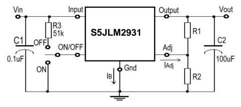
$V_{\text{OUT}} = V_{\text{REF}}^*(1 + R2/R1) + I_{\text{ADJ}}^*R2$
