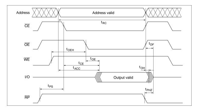
Read Timing Waveform (Byte Mode, Word Mode Switch)
