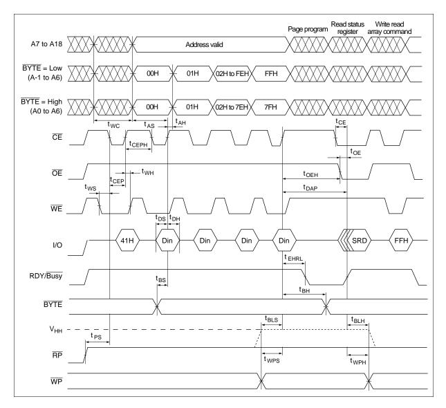
Write Timing Waveform for Erase Operations (WE control)
