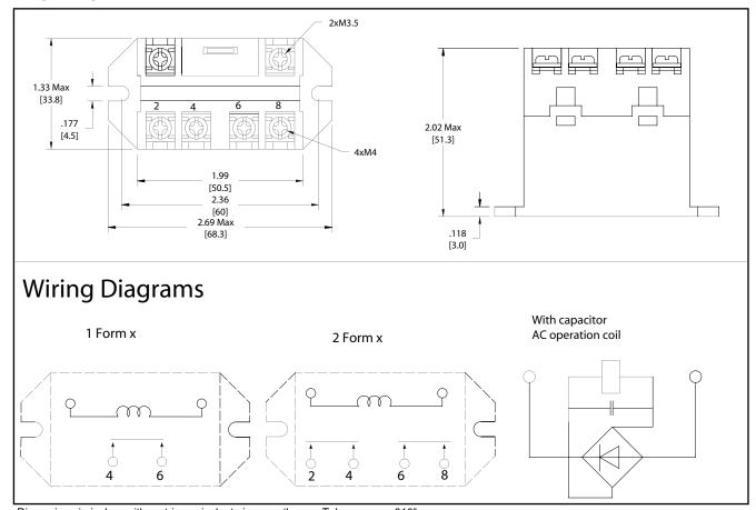
Dimensions in inches with metric equivalents in parentheses. Tolerance:  $\pm$  .010"
