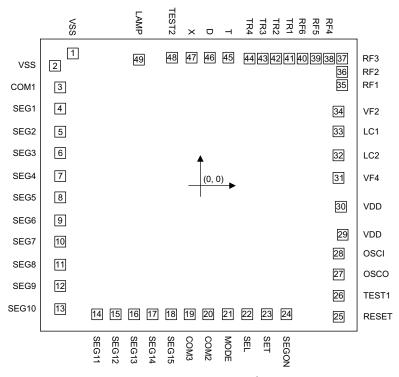
$\label{eq:chipsize: 2680 x 2460 ($\mu m$)$^2$} Chip thickness=12 mil$$^* The IC substrate should be connected to VSS in the PCB layout artwork.$
