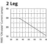
Ambient temperature (degrees C), measured 1 inch (25mm) below relay when mounted to DIN rail or a vertical, 1/8th inch thick aluminum panel surface. Airflow is unrestricted up and through the
