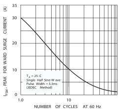
Fig. 3 Maximum Peak Forward Surge Current (per leg)
