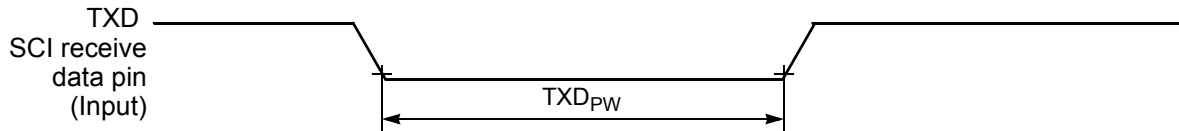
Figure 10-16 TXD Pulse Width
