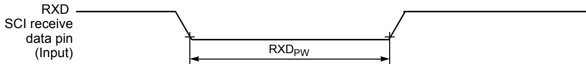
Figure 10-15 RXD Pulse Width
