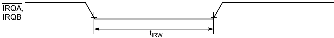
Figure 10-5 External Interrupt Timing (Negative Edge-Sensitive)
