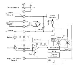
**NOTE #3:** pin #9 of CR3 model may be connected directly to the AUXILIARY input of a MAXI-AMP or Banner M Series module. It may also serve as the input to Banner CL series MAXI-AMPs or to Banner Plug Logic modules.
