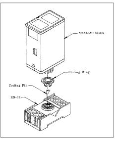
The RS-11 is supplied with a coding ring and pin (see diagram at right). This allows a MAXI-AMP to be keyed to fit only its own 11-pin socket. The pin is installed in one of the eleven slots in the RS-11, and the notch in the ring is aligned to slip over the pin. When the MAXI-AMP is removed from the RS-11, the coding ring stays with the MAXI-AMP base, while the coding pin remains in the socket.
