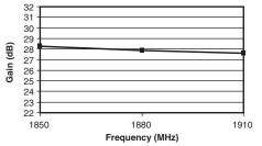
$\label{eq:RMPA1967} \begin{aligned} &\text{RMPA1967 3x3 US-PCS PAM} \\ &\text{Vcc} = 3.4\text{V}, &\text{Vref} = 2.85\text{V}, &\text{Vmode} = 0\text{V}, &\text{Pout} = 28\text{dBm} \end{aligned}$
