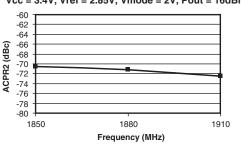
Low Power Mode (Vcc = 1.4V, Vref = 2.85V, Vmode = 2V, Pout = 16dBm)
