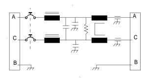
The ZG-1435-5B filter has been designed for systems operating under the requirements of MIL-STD-461C. If MIL-STD-461D or E are specified then part number ZG-1435-5BD should be specified. The difference is that the differential capacitor is repositioned on the line side in order to match the test configuration of 461D and E.
