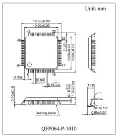
Note) The package of this product will be changed to lead-free type (QFP064-P-1010A). See the new package dimensions section later of this datasheet.
