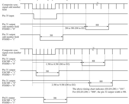
The pin 31 timing is synchronous with the pin 35 input timing. The above timing chart is just for reference
