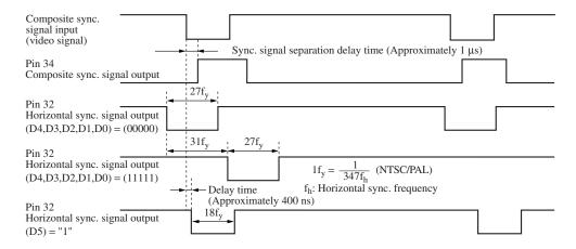
The delay time of pin 34 output to video signal is likely to vary according to an external constant connected to pin 46. For an external constant, the characteristics in weak electric field must be evaluated adequately.
