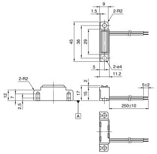
A ferromagnetic material such as iron with minimum dimensions of 45×12×1mm must be installed on mounting face A.
