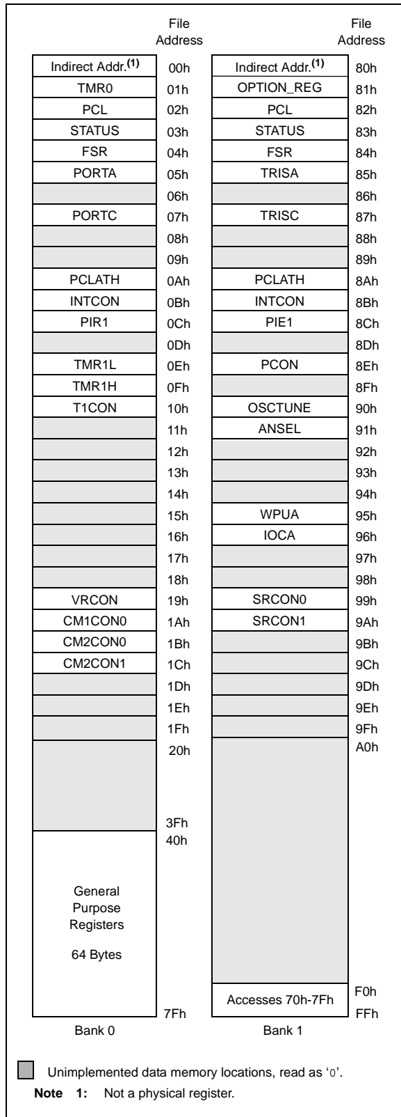
FIGURE 2-3: DATA MEMORY MAP OF THE PIC16F610/16HV610
