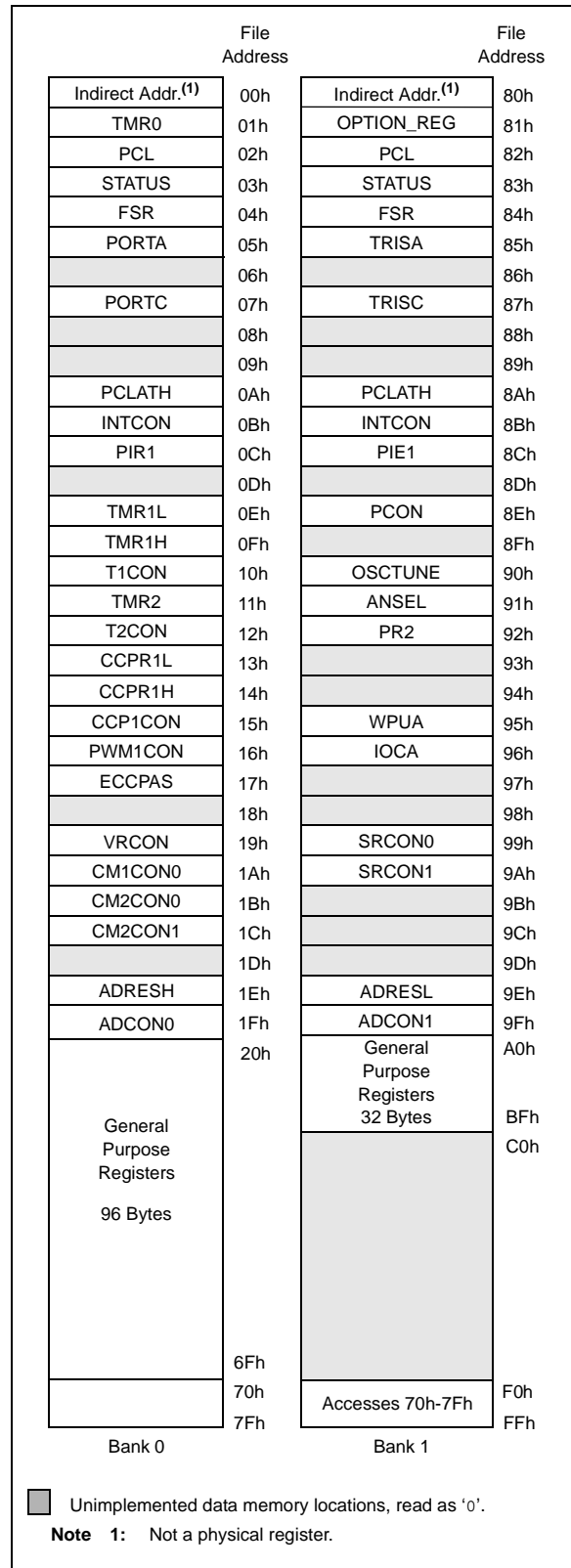
FIGURE 2-4: DATA MEMORY MAP OF THE PIC16F616/16HV616
