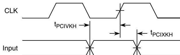
**Figure 26. PCI Input AC Timing Measurement Conditions**
