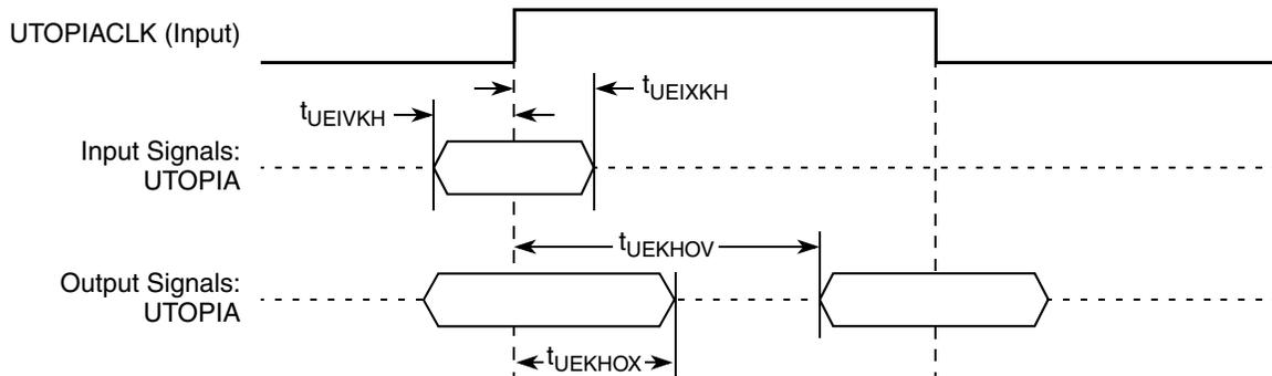
Figure 36. UTOPIA AC Timing (External Clock) Diagram
