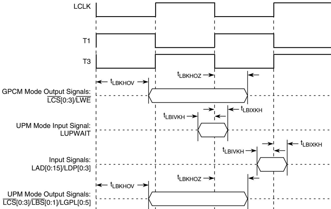
Figure 16. Local Bus Signals, GPCM/UPM Signals for LCCR[CLKDIV] = 2
