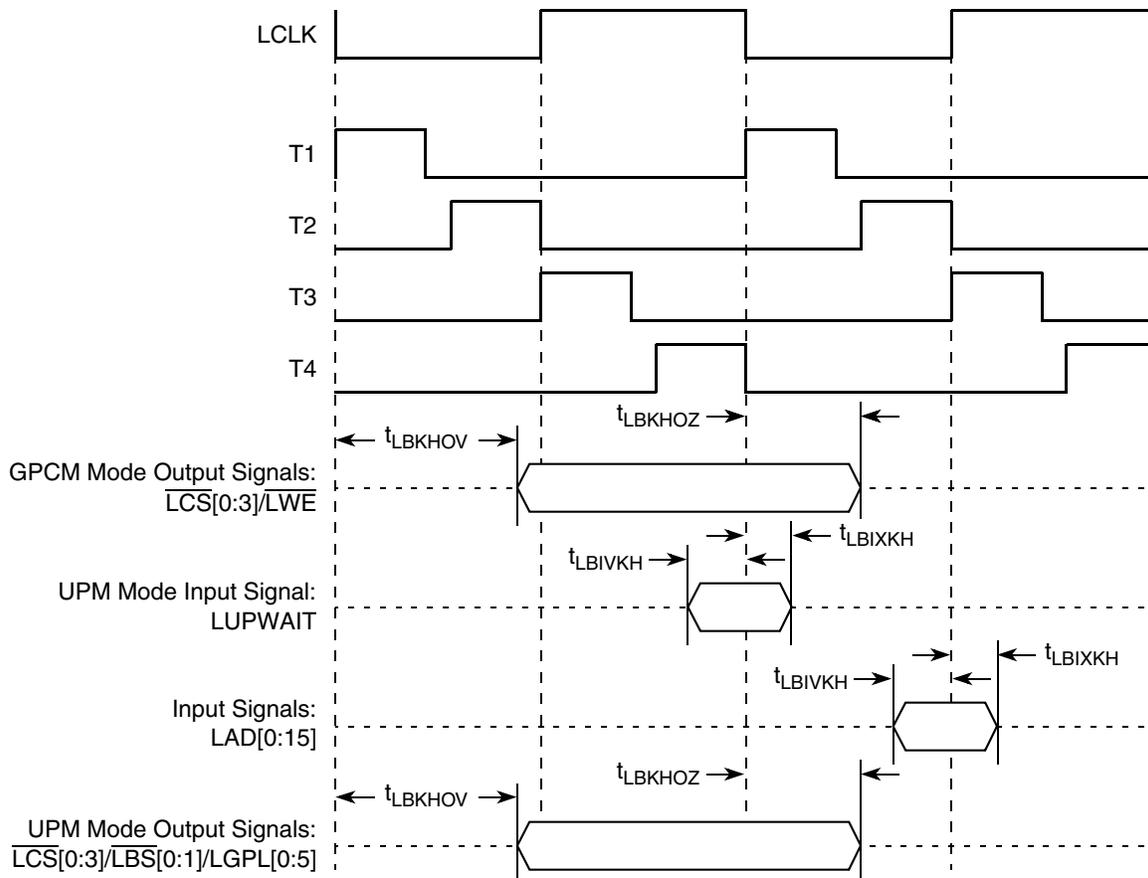
Figure 17. Local Bus Signals, GPCM/UPM Signals for LCCR[CLKDIV] = 4
