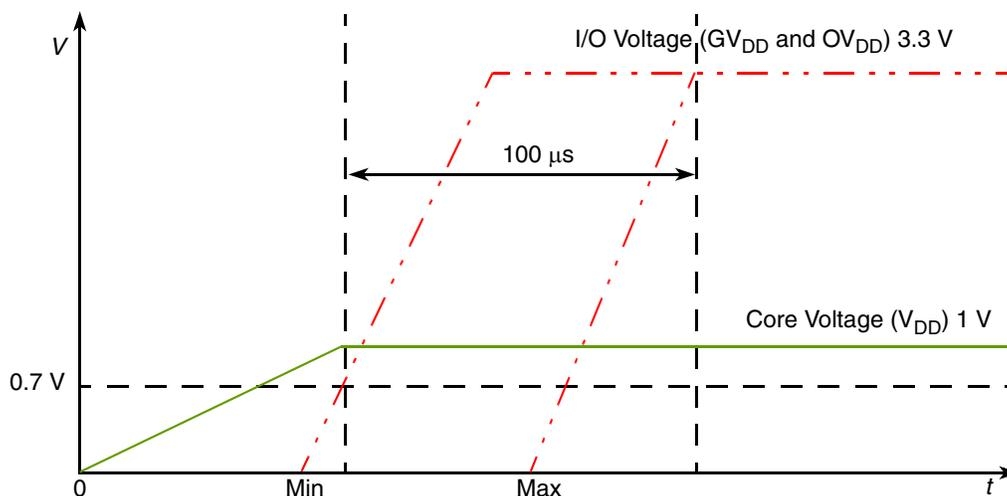
Figure 4. MPC8323E Power Sequencing
