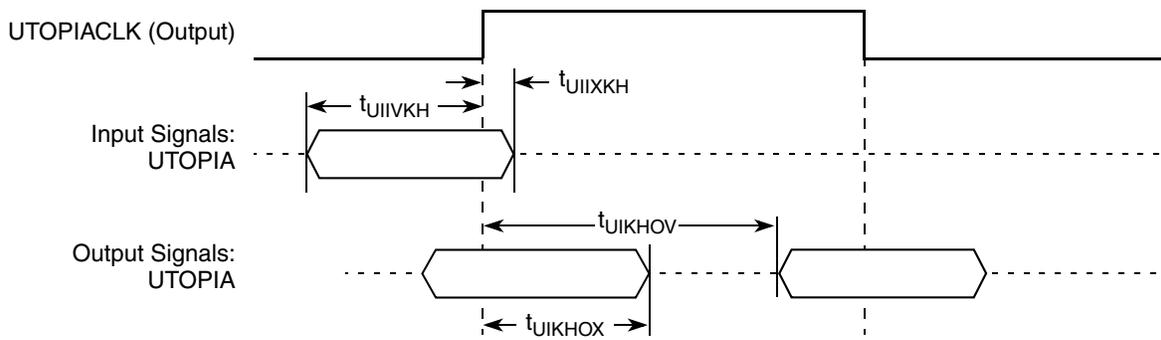
Figure 37. UTOPIA AC Timing (Internal Clock) Diagram
