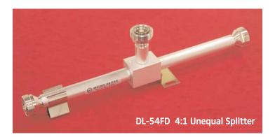
Microlab DL-D series Unequal Power Splitters unevenly split high power cellular signals in fixed ratios from 10:1 to 2:1 with minimal reflections or loss over the whole 800 - 2,500 MHz band. The multi section transformers ensure a good input VSWR and flatness across the band for both main and branch lines. To facilitate remote signal cable powering of amplifiers and control of antennas, DC - 2MHz continuity is maintained to both main and branch lines on all units to meet A.I.S.G. requirements.
