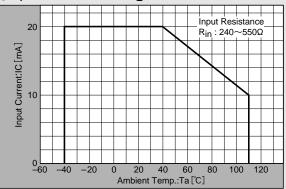
Note :  $\mathsf{R}_{\mathsf{in}}$  of Hall element decreases rapidly as ambient temperature increases. Ensure compliance with input current derating curve envelope, throughout the operating temperature range.
