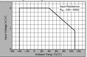
Note : For constant-voltage drive, stay within this input voltage derating curve envelope.
