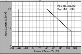
Note: Rin of Hall element decreases rapidly as ambient temperature increases. Ensure compliance with input current derating curve envelope. throughout the operating temperature range.
