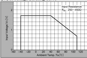
Note: For constant-voltage drive, stay within this input voltage derating
