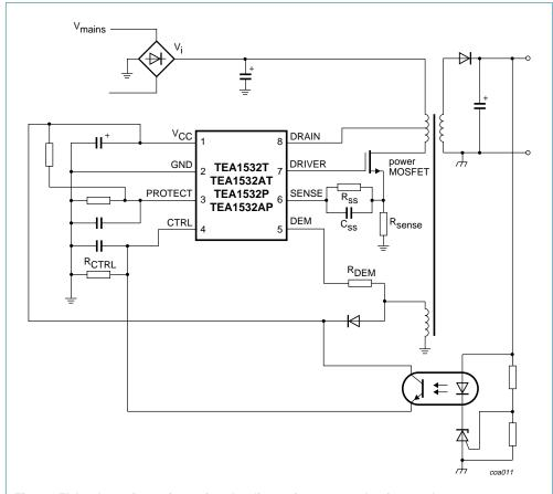
Fig 10. Flyback configuration using the discontinuous conduction mode
