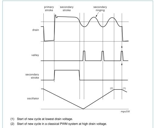
Fig 8. Signals for valley switching
