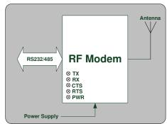
The RF modem can be configured to scan the radio link for activity and verify it is free before transmission thereby avoiding data collisions.
