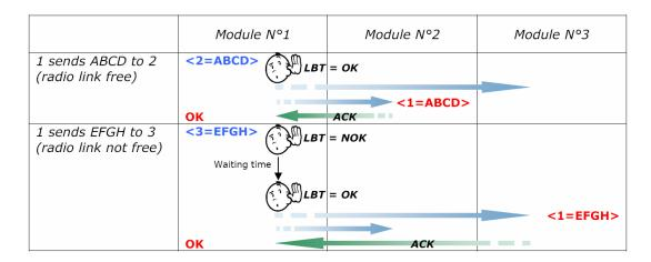
In this mode the RF modem can be configured to scan the radio link for activity and verify it is free before transmission (listen before talk) thereby avoiding data collisions.
